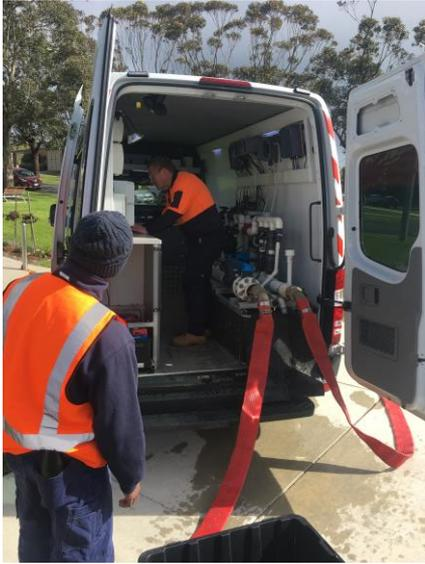
Specialist contractors hook equipment up to the water main to sample and test water quality and cleanliness of pipes. Using this data, South Gippsland Water will plan maintenance and cleaning programs.
