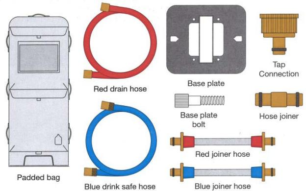
**Step 2:** Remove the base plate from the front pocket of the carry bag.
