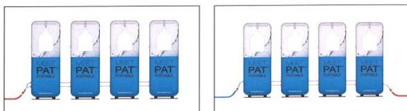
**Step 9:** Once the hoses are connected, turn on the water supply. Check for leaks.
