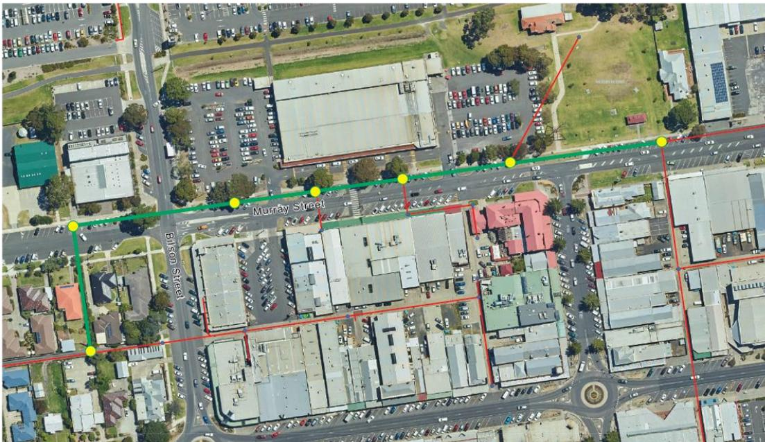
Key: — Existing Sewer Pipe — Sewer Pipe Upsized ● Manhole/Excavation
