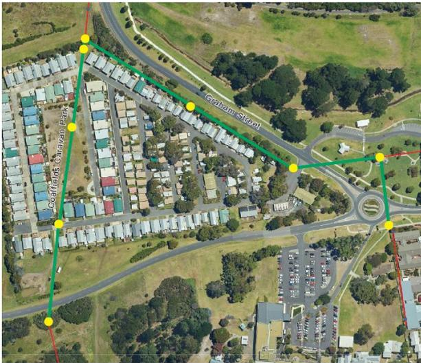
Key: — Existing Sewer Pipe — Sewer Pipe Upsized ● Manhole/Excavation
