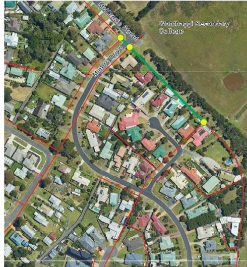
Key: — Existing Sewer Pipe — Sewer Pipe Upsized ● Manhole/Excavation
