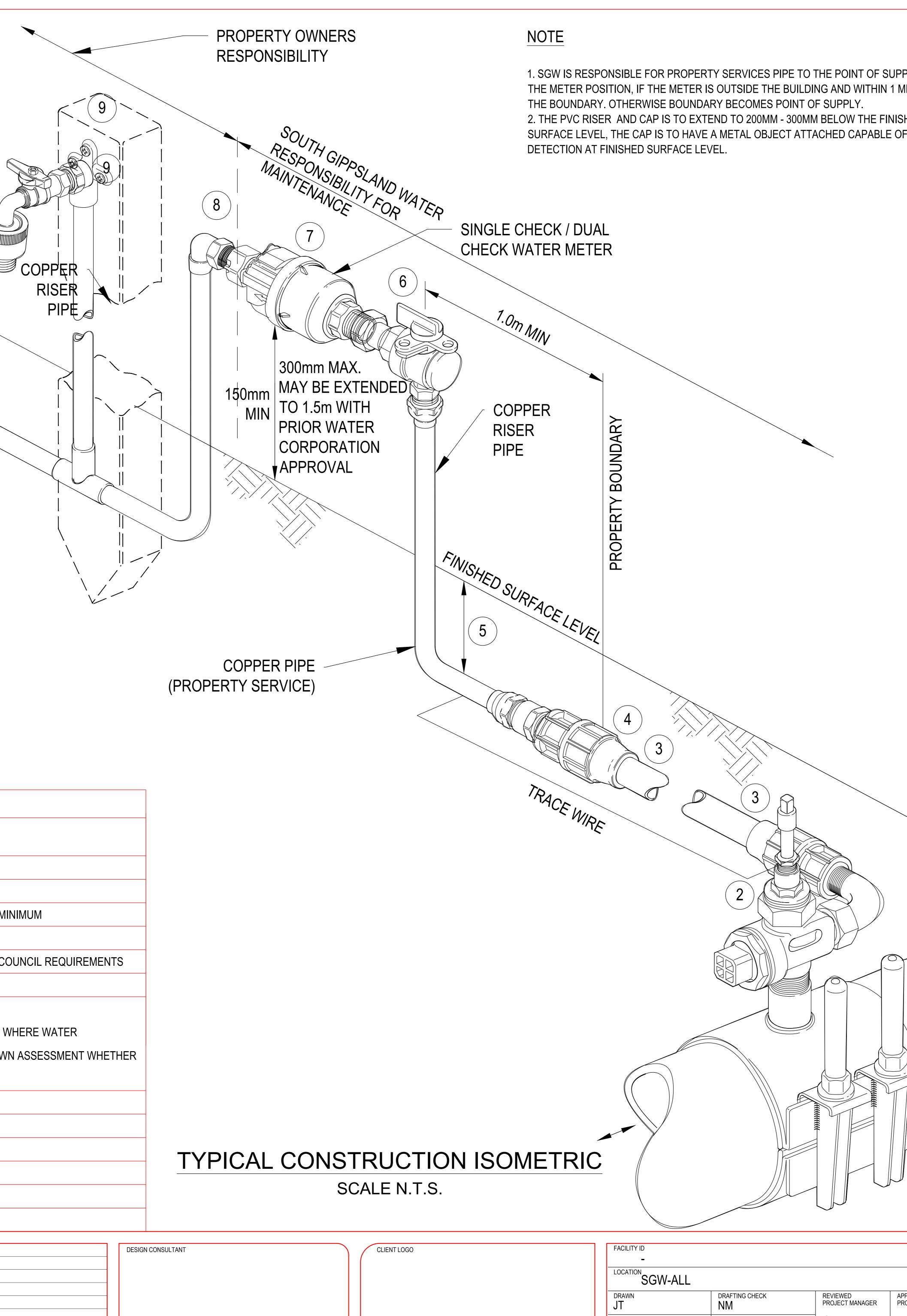
1. SGW IS RESPONSIBLE FOR PROPERTY SERVICES PIPE TO THE POINT OF SUPPLY THAT IS THE METER POSITION, IF THE METER IS OUTSIDE THE BUILDING AND WITHIN 1 METER OF 2. THE PVC RISER AND CAP IS TO EXTEND TO 200MM - 300MM BELOW THE FINISHED SURFACE LEVEL, THE CAP IS TO HAVE A METAL OBJECT ATTACHED CAPABLE OF METAL
