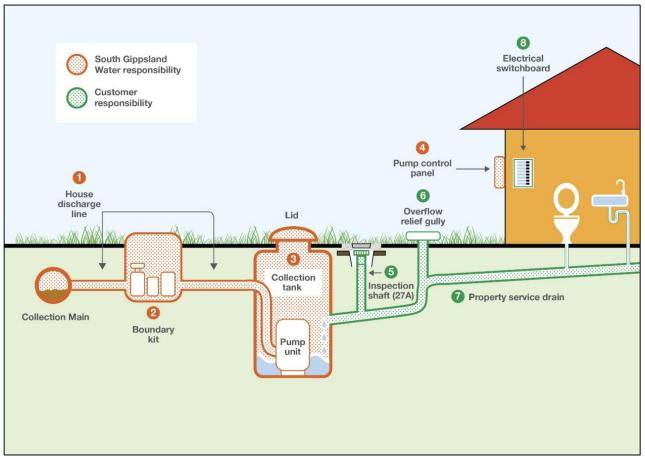
Figure 3: Pressure Sewer Infrastructure Ownership Diagram
