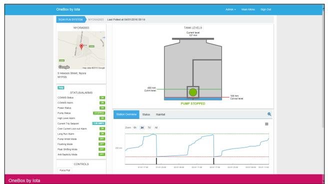
Figure 2: South Gippsland Water One Box SCADA Software
