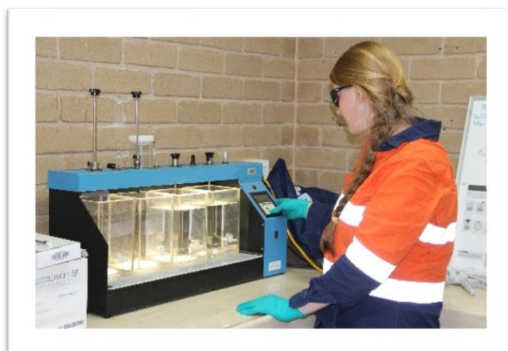
Photo: Water Treatment Plant Operator conducts a jar test
