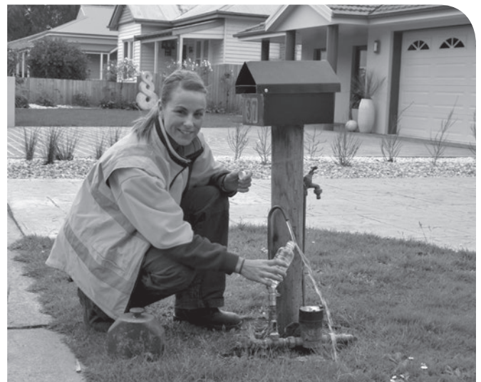
Megan Hoskins collecting water samples for testing as part of the water quality monitoring program.
