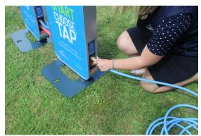
Step 7: Connect the red drain hose to the red drain outlet. The drain outlet can be connected to either side of the unit.
